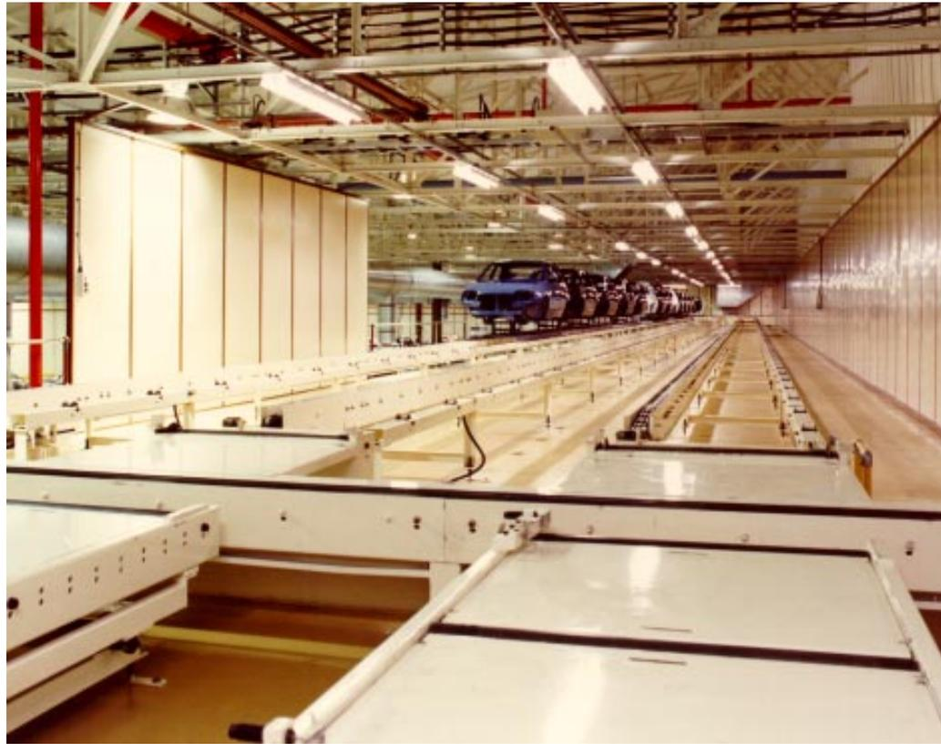
***Webb's belt skid conveyor systems are clean, quiet, compact and easily maintained. Components are assembled in a modular configuration to minimize field installation.***
